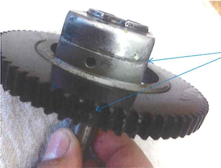
Gear (P/N GE52198) is pitted & has one gear tooth damaged. This part is rejected.
